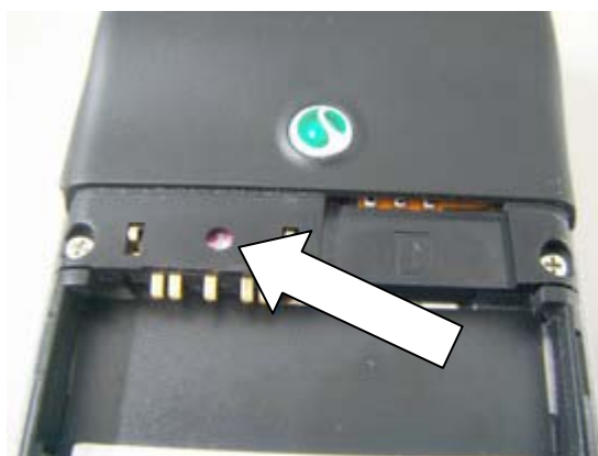
Location of the Liquid Intrusion Indicator. (Remove battery cover)
